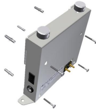
Figure 8: Installation of the fixed support
